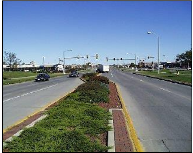
Figure 2 – Center median with left turn lanes
