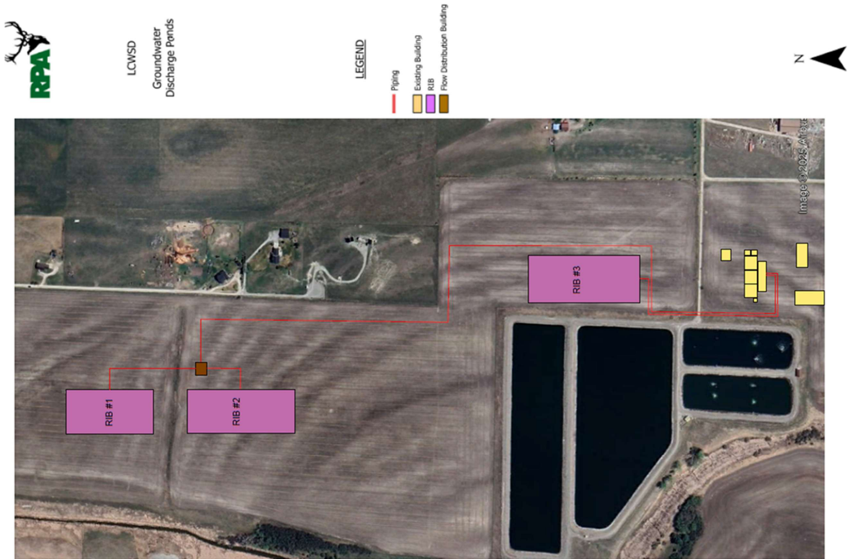
Figure 3. Phase 2 Wastewater Improvements Layout – RIB Locations
